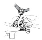
1 Align the two triangles and clipse the cushion on the frame.
